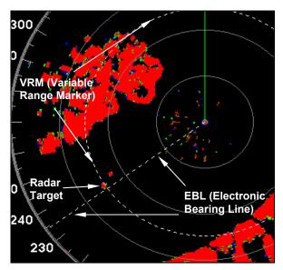
This is a zoomed in view from the previous image, clearly showing the radar target, Variable Range Marker and Electronic Bearing Line.
